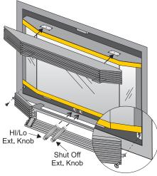
3) Open the bottom louver. Pull the Burner ON/ OFF control box from inside the bottom of the fireplace. Using the 2 screws on the louver, secure the control box in place.
